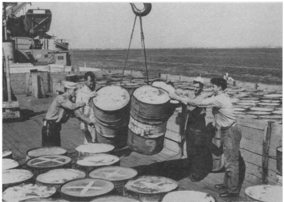
RADIOACTIVE WASTES READY FOR DUMPING IN OCEAN —Two sailors and two health physicists from the Brookhaven National Laboratory, Upton, N. Y., stow low level radioactive wastes aboard a Navy LST for disposal at sea. This Brookhaven picture was made at Floyd Bennett Field, Brooklyn.
