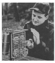
posable propane gas cylinder, the portable burner, shown in the photograph, provides a cooking effect comparable to that attained with charcoal or with resistant-wire type electric broilers. It is about the size of a large lunch pail and weighs nine pounds with fuel.
