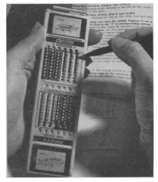
the reverse side is a device for quick addition or subtraction up to 999,999. The aluminum and brass adding device is operated by a stylus contained in the rule's leather case.
