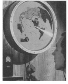
wall or mounted directly on the control table. The light wedge, ten degrees wide at the edge of the indicator, moves on the map as the antenna rotates, and shows beam direction and width.
