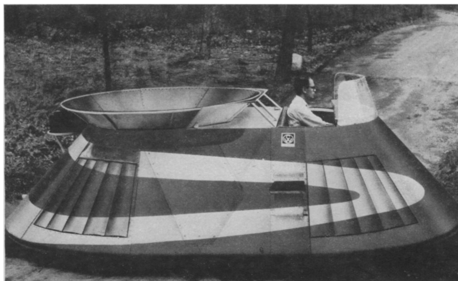
AIR-CAR—Using a conventional type piston engine of from 50 to 200 horsepower, the Curtiss-Wright Air-Car lifts itself from six to 12 inches off the ground. It has no conventional wheels, axles, brakes, clutches, transmission or frame. Low pressure, low velocity air supports and propels the vehicle over unobstructed ground or water.
