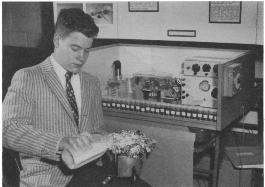
DO-IT-YOURSELF RADIATION DETECTOR —Robert Schooley, 17-year-old high school junior, pours milk into a device he built and used to measure the total radioactivity of milk in the Washington, D. C., area. He found that the radioactive content of milk fluctuates.
