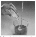
Into a liquid triglyceride such as cottonseed oil put a small percentage of monoglyceride made from any saturated fat.
