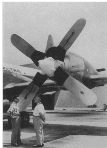
ROUND-TIP PROPS —Made of solid dural, an alloy of aluminum, these 13½-foot propellers with round tip blades are geared to Allison turbine engines. The round tip blades, described as a new design, are being tested by Lockheed Aircraft Corp. in Burbank, Calif.
