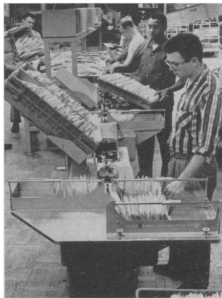
FACER-CANCELER — A new machine, capable of facing and canceling letters up to 500 a minute, is one of the devices breaking postal bottlenecks.
