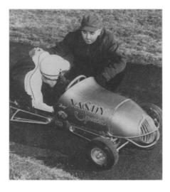
of cpoxy and glass fiber. The racer, available either as a complete car or in kit form, has individual wheel torsion suspension, an adjustable steering column, friction shock absorbers, and a tubular aircraft type frame.
