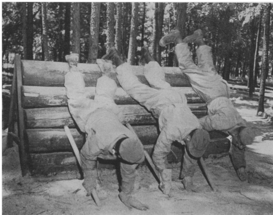
PAPER UNIFORMS —These soldiers, clambering over a training obstacle, are testing experimental paper throw-away uniforms. This U. S. Army photograph, taken at Fort Lee, Va., shows only one of the rigorous tests to which the uniforms are being subjected.
