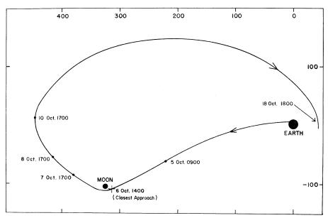
RUSSIAN MOON—This diagram of the artificial satellite launched by Russian scientists and now circling the earth and its moon was prepared by the Smithsonian Astrophysical Observatory, Cambridge, Mass. Lunik III, as the satellite is called, takes an estimated 13 days to make a complete circuit of its orbit. Its perigee, or nearest point to the earth, is estimated at 24,853 miles; apogee is 292,000 miles. Lunik III's life expectancy is described as "unlimited."
