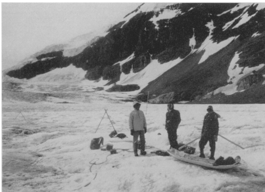
RADIO FREQUENCY EXPEDITION —A team from the National Bureau of Standards' Central Radio Propagation Laboratory encounter bad weather on a glacier in northern Canada as they measure the complex conductivity of ice over the radio frequency range from 20 to 200 kilocycles. This expedition is illustrative of many that are made to remote places by CRPL personnel in the NBS program of radio propagation research.
