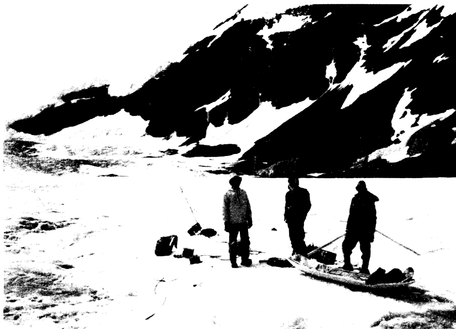
RADIO FREQUENCY EXPEDITION —A team from the National Bureau of Standards' Central Radio Propagation Laboratory encounter bad weather on a glacier in northern Canada as they measure the complex conductivity of ice over the radio frequency range from 20 to 200 kilocycles. This expedition is illustrative of many that are made to remote places by CRPL personnel in the NBS program of radio propagation research.
