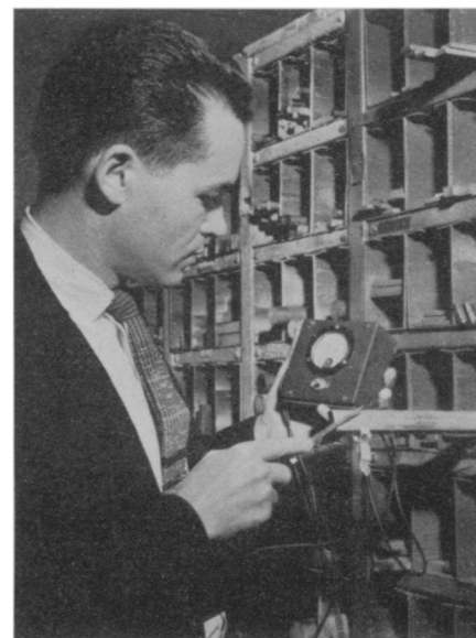
METAL SORTER —A "metal sorter" has been invented by George Martin of the General Electric Company that identifies different look-alike metals commonly used in nuclear reactors. The device is basically a milliammeter with a single clamp-on lead and another lead with a carbon steel file on the end.
