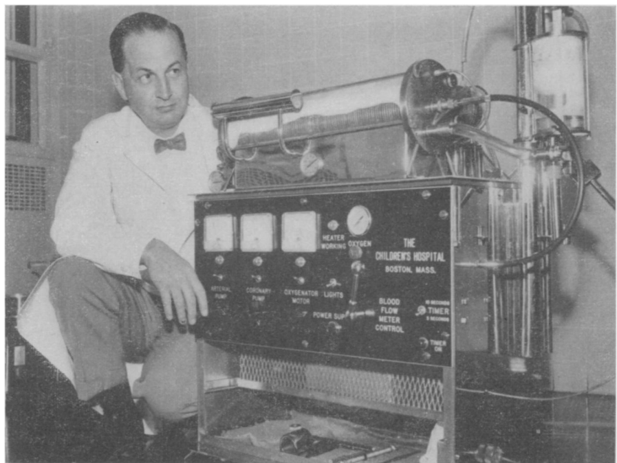
MECHANICAL HEART AND LUNG —This machine has assumed the duty of both the heart and lungs of more than 250 patients undergoing a heart operation. The machine was developed by Dr. Robert E. Gross of Children's Hospital, Boston.
