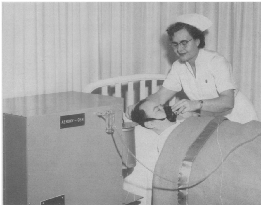
OXYGEN FROM THE ROOM —This transportable oxygen unit draws air from the atmosphere, filters out contaminants, extracts oxygen and furnishes this gas to the patient. Developed by Aerojet-General Corporation's Chemical Division, Azusa, Calif., it is expected to be widely used in hospitals and ambulances.
