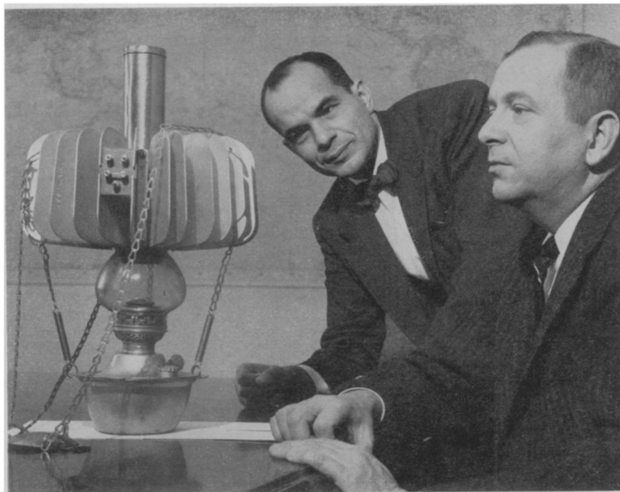
THERMOELECTRIC GENERATOR —The Russian thermoelectric generator converts heat from a kerosene lamp into electricity for radios in remote Asian areas. The generator is examined by J. Donald Rauth (right) and Dr. Mostafa E. Talaat (left), both of The Martin Company, Baltimore, Md., that used similar principles in conjunction with a radioisotope heat source.
