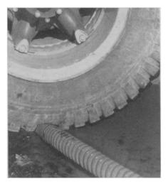
seen in the photograph, is constructed to rebound to full diameter even after being run over by a heavy dump truck.
