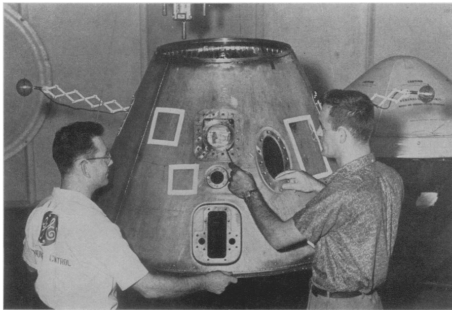
RE-ENTRY VEHICLE —This experimental missile re-entry vehicle of the Air Force Research and Development Command's Cambridge Research Center contains instruments for measuring meteor sizes and electrical energy in space. Engineer Joseph Frissora of Geo-Sciences, Inc. is pointing to his self-designed meteor detector. The "ears" on each side of the vehicle measure ion densities and the electrical potential of the re-entering vehicle.
