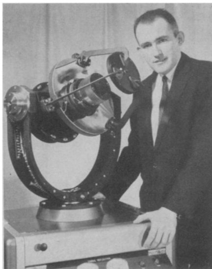
INFRARED SCANNER —This 50-pound gyrosopic far infrared scanner, made by the Martin Company's Baltimore Division, will be used for missile guidance or interplanetary navigation. Project engineer Irving E. Distelhorst's face is reflected in the scanner's primary mirror.
