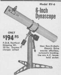
Finest American-made 6-inch reflector in its price rangel Save \$100 or more, yet get all these fine features: f/8 6-inch mirror accurate to ½ wave \* electric drive \* 3 matched eyepieces (75X, 150X, 343X) \* 6x30 Achromatic finderscope \* Heavy-duty mount with setting circles \* Rack & Pinion eyepiece holder \* Rotating tube \* Sturdy lightweight tripod.
