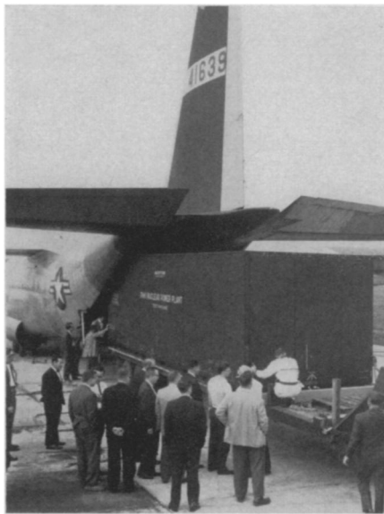
15 NUCLEAR TONS —A test package representing one section of a nuclear power plant, weighing 15 tons, is loaded into a C-130A aircraft at The Martin Company's airport in Baltimore. The plant is being built by Martin for the U. S. Atomic Energy Commission and will be installed next year at Sundance Air Force Station, Wyoming.
