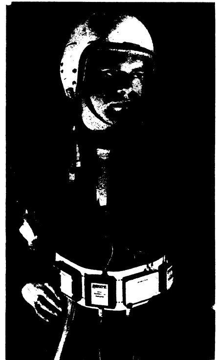
MINIATURIZED INSTRUMENTS —Simultaneous recording of body functions is possible with the instruments worn on the belt of the flyer. Developed by scientists at the Boeing Space Medicine Section, Seattle, Wash., the instrument belt is adaptable to space flight.
