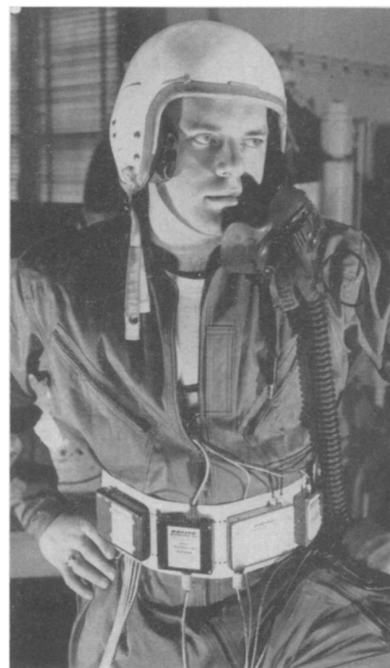
MINIATURIZED INSTRUMENTS —Simultaneous recording of body functions is possible with the instruments worn on the belt of the flyer. Developed by scientists at the Boeing Space Medicine Section, Seattle, Wash., the instrument belt is adaptable to space flight.
