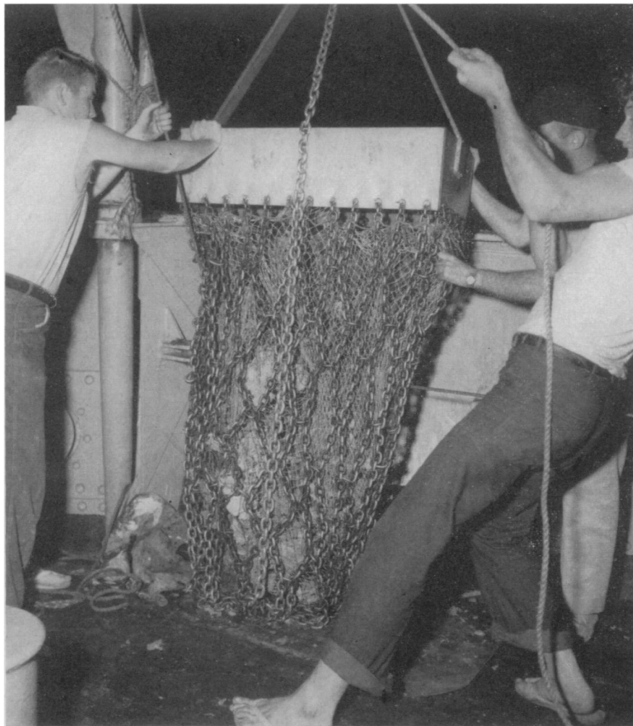
DREDGING THE SEA —Survey workers hoist a large haul of rocks aboard the Explorer during night dredging operations. The ship recently made a 79-day research cruise, the largest oceanographic undertaking by the U. S. Coast and Geodetic Survey in 70 years.
