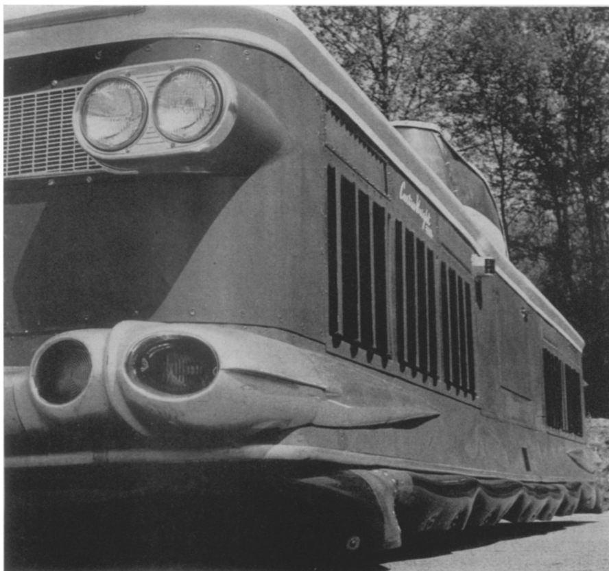
RIDING ON AIR —The Curtiss Wright Air Car rides on a "cushion" of air that is directed straight down to the ground by a urethane skirt, a highly abrasion-resistant material. The United States Rubber Co. developed the skirt, which also protects the vehicle's undersurface.
