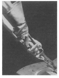
aluminized asbestos backs and thumbs. The gloves are long enough to protect
