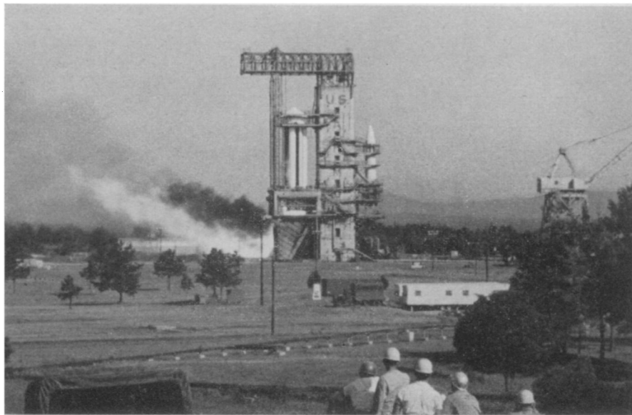
GOING NOWHERE —The free world's mightiest booster, the Saturn, roars and thunders but is held to the ground in a test of its eight engines. Additional hardware, such as skirts and pressurization equipment, are now being added for a second series of static tests. Then—flight.
