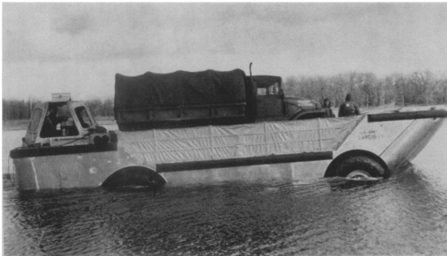
THE LARC-15—After a test run on land and water from Kalamazoo to Chicago, this aluminum "cargo lighter" is ready for business. The combination cargo and personnel carrier for ship-to-shore deliveries was developed by the U. S. Army Transportation Research Command. The LARC-15 derives its name from "Lighter, amphibious, resupply, cargo."
