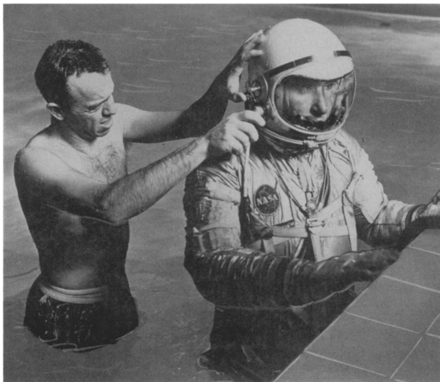
ASTRONAUT IN PRESSURE SUIT —Astronaut Walter Schirra tests a full pressure suit for water tightness in a swimming pool. He is assisted by fellow Astronaut Alan Shepard. The suit, manufactured by B. F. Goodrich Company, was developed for the seven Astronauts for NASA's Project Mercury manned orbital flight program.
