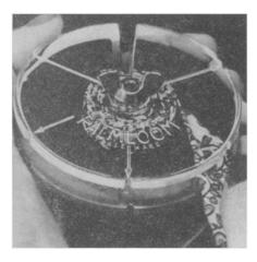
of remnant materials are wound up and then put through slots in the loom, shown in the picture. The circular pieces produced may be sewn together into larger items.
