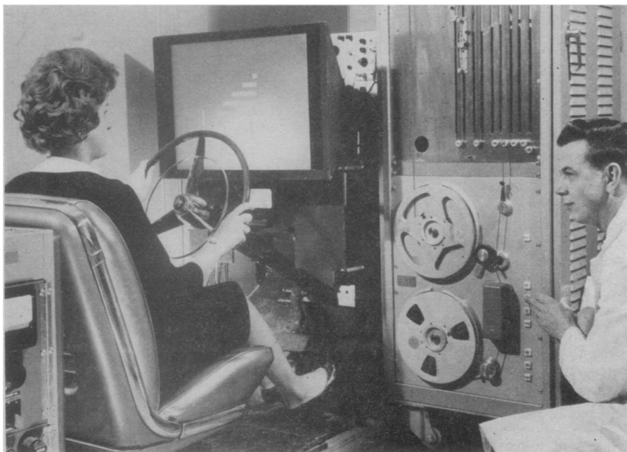
SYNTHETIC CAR —Developed by General Motors Research Laboratories to study interaction of driver and vehicle controls, this analogue driving simulator gives the illusion of turns in the road, and the driver steers to follow.
