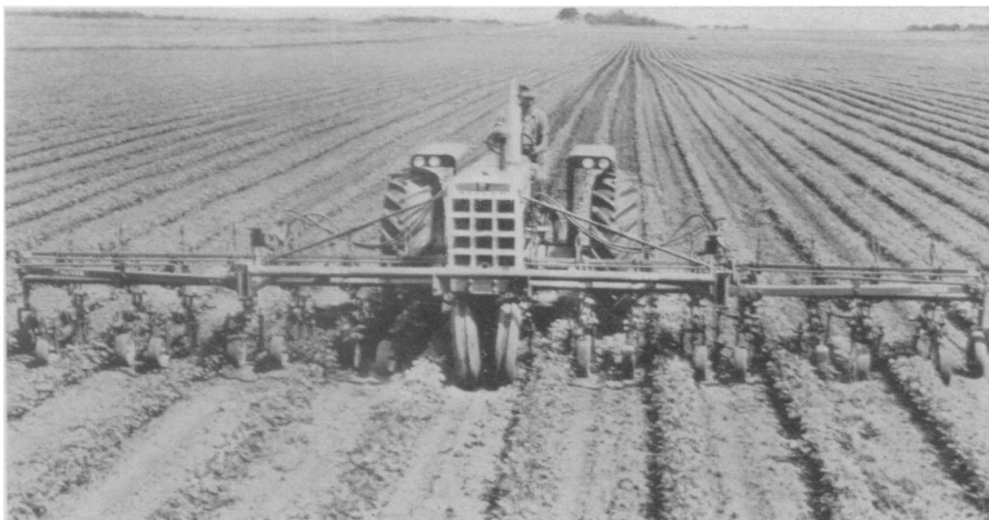
EIGHT-ROW-CULTIVATOR —Primarily used for soybeans and corn, a tractor-mounted cultivator, developed by Oliver Corporation of Chicago, handles eight rows instead of the usual four.
