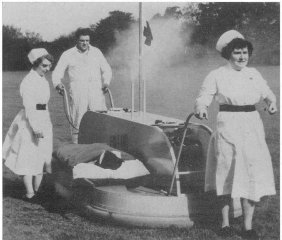
RIDE ON AIR —A stretcher-carrier, developed by Folland Aircraft, Southampton, England, gives a joltfree ride to patients. The vehicle is supported by a chamber of air cushions.
