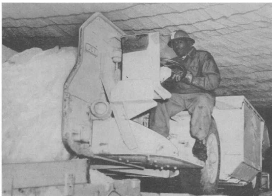
UNDER ICE —Under the ice cap 700 miles from the North Pole in northwest Greenland, shuttle cars pick up loads of ice from area where a mechanical miner is digging a large excavation for year-round storage of materiel and housing of personnel in the Arctic. The shuttle cars run on batteries of a type invented by Edison, made by The Electric Storage Battery Company, Philadelphia.
