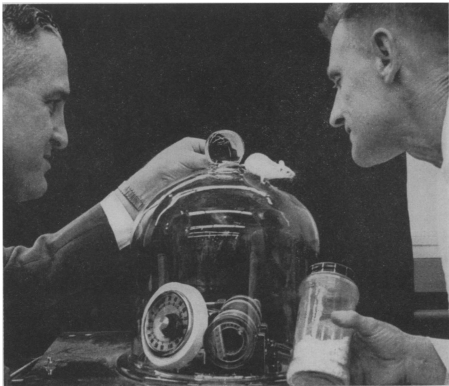
CHEMICAL OXYGEN SUPPORTS MOUSE —A house mouse was supported for 80 hours in a cell where its only source of oxygen at a simulated 75,000 feet altitude was potassium superoxide . Stan Hall and C. C. Simms examine the mouse at Lockheed Missiles and Space Company, Sunnyvale, Calif., where the experiment was performed.
