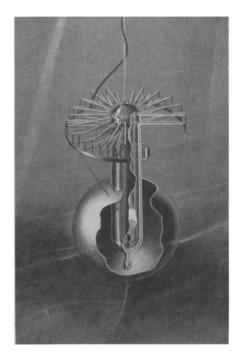
POWER IN THE DEEP—Undersea atomic plant will be developed by General Dynamics Corporation, San Diego, Calif., as thermoelectric power source for naval units. Tubes at top change reactor heat to electricity.
