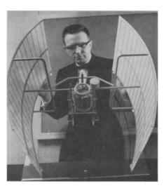
NUCLEAR POWER SYSTEM—A nuclear thermoelectric system that could power instruments gathering scientific data on the moon has been developed by the aerospace electrical department of Westinghouse, Lima, Ohio. Niles F. Schub shows a model of the system using spontaneous decay of a radioisotope to produce heat which is converted into electricity. The curved shields are waste heat radiators.
