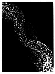
NEW TWIST—Graphite cloth, magnified 150 times, shows more than 1,400 filaments per twist. The fabric, produced by National Carbon Company, a division of Union Carbide Corporation, New York, is being combined with plastic resins in the molding of missile and rocket motor components such as nose cones.
