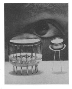
varying light intensities. Available in four basic sizes, the cells can be used to turn on street lights, adjust lens opening of cameras, for blood pressure gauges, burglar alarms, headlight dimmers, radiation detectors and many other devices.
