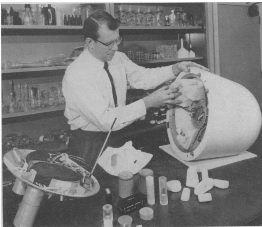
LOADING BIOS I —A NASA engineer places plastic foam in Bios I as padding for the small capsules containing biological experiments.
