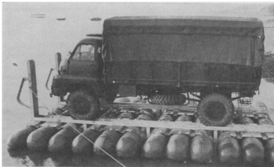
NYLON RAFT —Weighing slightly more than 2,000 pounds, this nylon and aluminum raft can support a load 10 times its weight. It was designed for the British Army and is now undergoing tests in the Far East. A series of rafts can be joined together to form a pontoon bridge.
