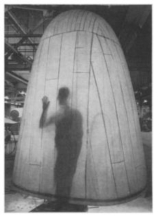
DISJOINTED NOSE—An inspector's shadow diffuses in a ghost-like shape as light shines inside an airplane nose section. The radome, contructed of strips of fiber glass honeycomb covered with a resin-impregnated glass fiber skin, is being constructed by Goodyear Aircraft Corporation to house antenna equipment for a modified version of the KC-135 jet tanker. The structure which is nine feet long and seven feet wide at the base is designed to withstand speeds approaching that of sound.
