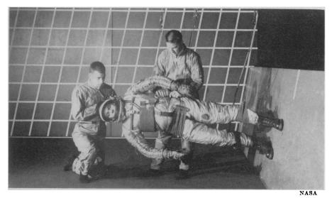
A WALK AT ONE-SIXTH G-A system of slings supports the weight of a man and allows him to walk and jump under conditions simulating the gravitational forces on the moon's surface at the Langley Research Center of the National Aeronautics and Space Administration.
