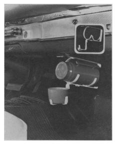
is mounted under the dashboard with a single clamp. No holes need to be drilled. Useful to travelers with young children or to long-distance truck drivers, the holder will accommodate a thermos bottle of quart size or smaller. A removable cup holder keeps the filled cup upright and secure. Made of lightweight aluminum, the holder is also useful for keeping other items within convenient reach.
