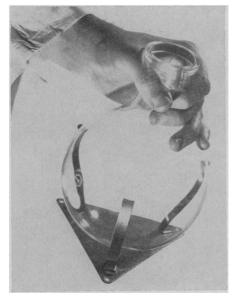
round-bottom flasks consists of a triangularshaped stainless steel base with a springy stainless steel finger at each corner. To use, the flask is pushed down between the fingers which hold it tightly. The holder allows the laboratory workers to move the flask from place to place with only one hand, not possible when using the traditional cork rings. The holder comes in various sizes.
