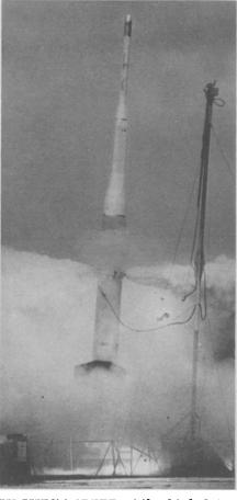
HIGHEST SPEED-The high-flying Lockheed X-17 blasts off on its journey into the ionosphere as spin rockets on its side, which will drop off after the launching, give it a stabilizing twirl. The Department of Defense reports the X-17, developed by Lockheed Missile Systems division in Van Nuys, Calif., has reached the highest speed ever achieved by an instrumented vehicle. The three-stage missile is described as the biggest and most powerful in existence using all solid propellants.
