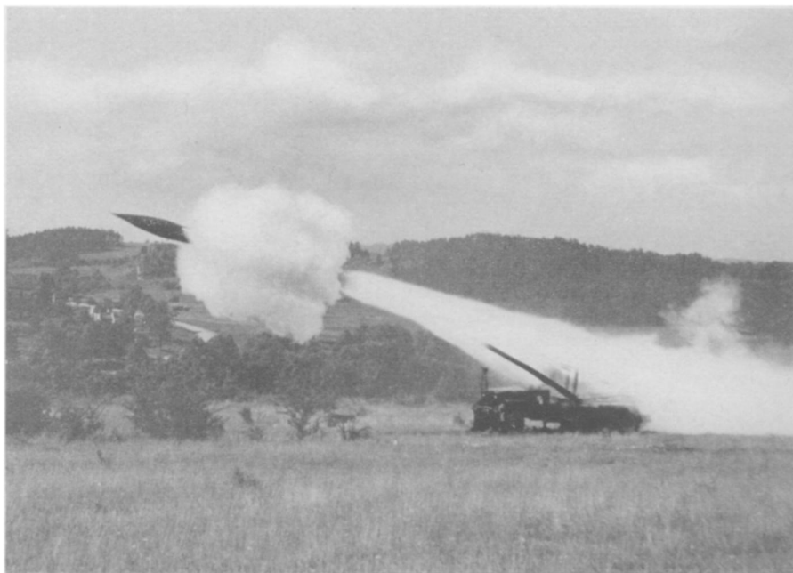
LAUNCH SOLID PROPELLANT ROCKET —An Honest John free-flight artillery rocket is fired at a U. S. Army training area in southern Germany. A solid fuel provides all the energy needed to send this 27-foot-long, 6,000-pound rocket to a target up to 15 miles away. The solid fuel is safer and more dependable than the liquid fuels formerly used in similar weapons.
