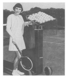
ball server delivers the balls at five-second intervals and can take 40 balls at one loading. The ball thrower can be set and reset for speed and direction.
